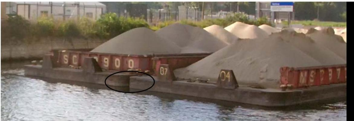
Figure 12. Picture of two barges traversing the electrical barrier with the square ends in the front of the barge configuration. The circle denotes the small void space that two live fish swam into and became entrained past the barrier.
