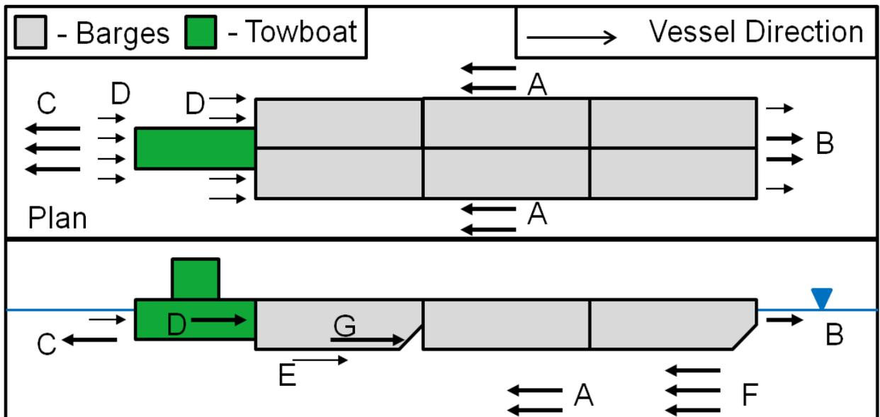
Figure 3. Water motions around tows moving left to right in confined channels. A = return velocity, B = bow wave, C = propeller jet, D = wake flow, E = flow in boundary layer along hull, F = displacement flow at bow between hull and channel bottom having short duration and G = pocket recirculation. Figure created by ERDC-CHL.
