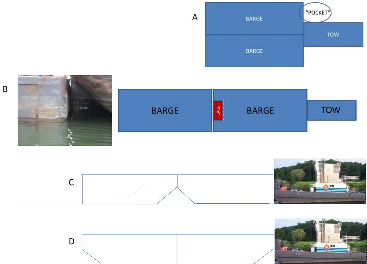
Figure 10. Schematics of four barge configurations used for voltage measurements at junctions and for fish interaction evaluations. A = Parallel barge configuration in which the tow boat is centered on the two barges. As the barges move forward a “pocket” eddy of water forms in the wake flow that can move debris forward with the barge. B = rake-to-box configuration. C = rake-to-rake configuration. D = rake-to-tow configuration.
