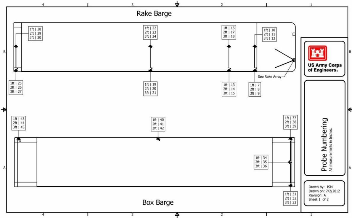
Figure 6. Sensor array locations and numbering for the rake and box barges.
