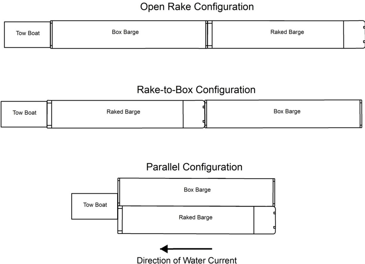
Figure 8. Barge Testing Configurations
