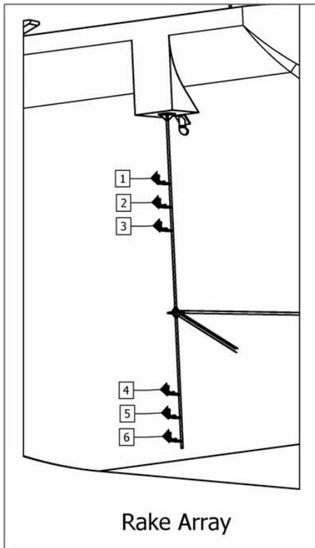
Figure 7. Rake array locations and numbering
