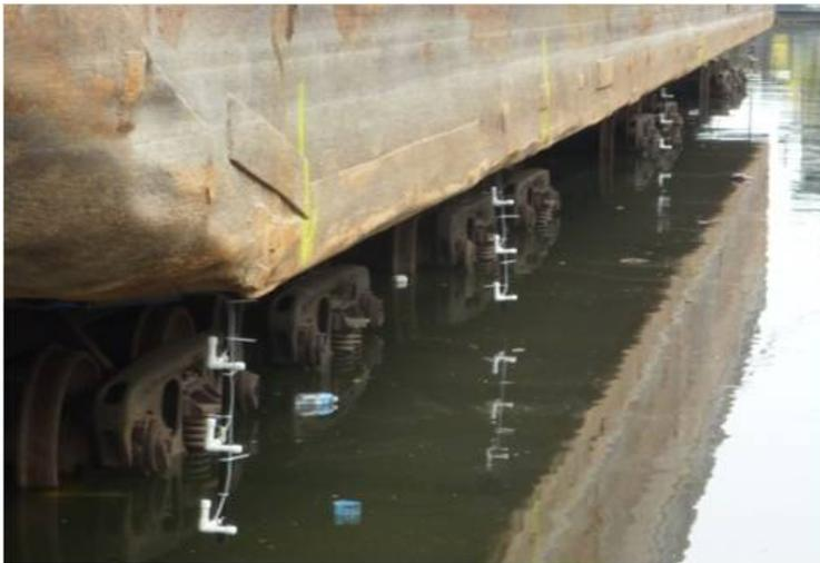
Figure 5. 3 Dimensional probe arrays along the bottom edge of rake barge in dry dock.
