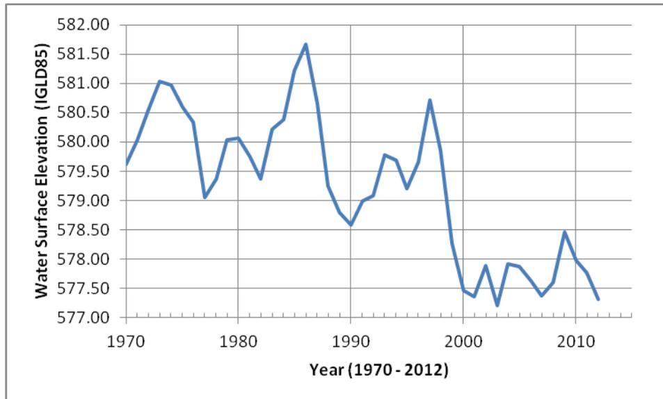
Figure 2.2 Calumet Harbor Gage Data – Annual Means for Period of Record
