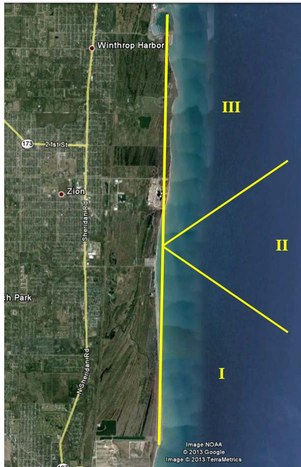
Figure 2.3 Definition of Site Wave Angle Classes
