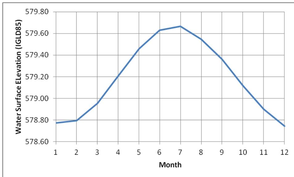
Figure 2.1 Calumet Harbor Gage Data – Period of Record Monthly Mean
