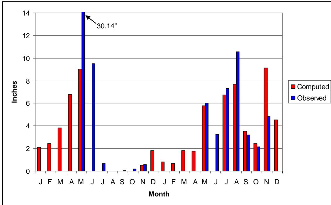
Figure 9. Comparison of Computed Runoff to Measured Flows in Basin D.
