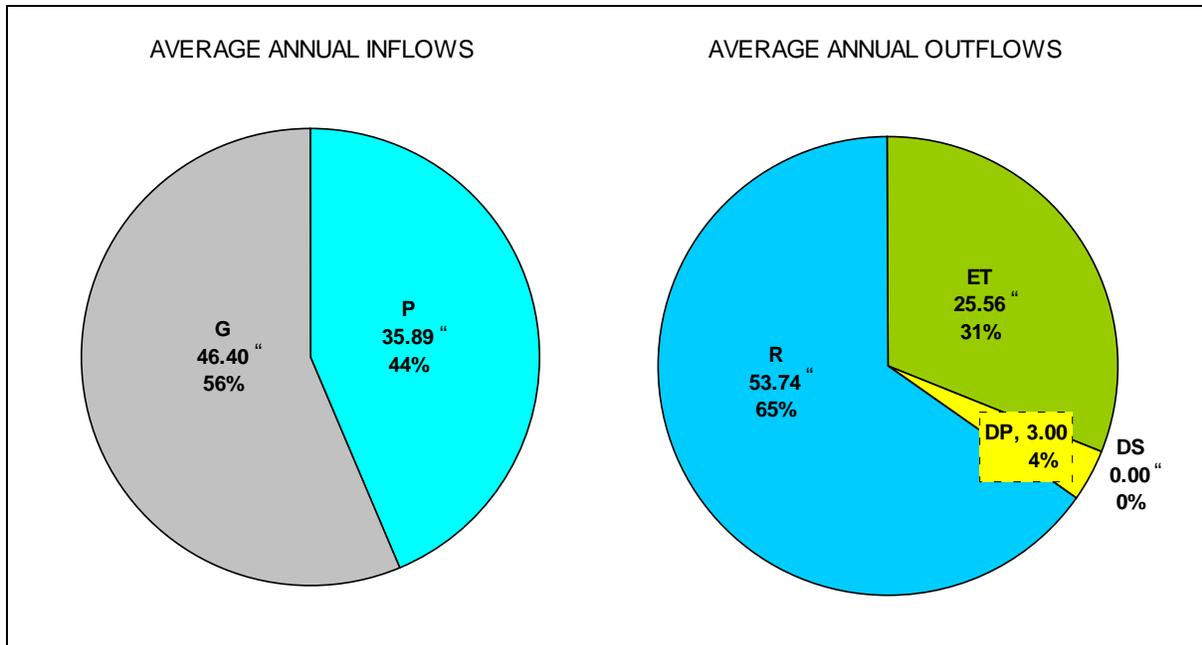
Figure 7. Water Balance Results, West of Railroad Tracks.
