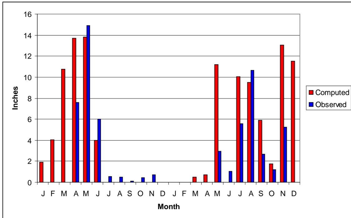
Figure 8. Comparison of Computed Runoff to Measured Flows in Basin B.
